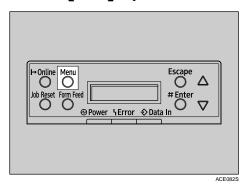
Press the [▲] or [▼] key to display "Sample Print", and then press the [# Enter] key.
